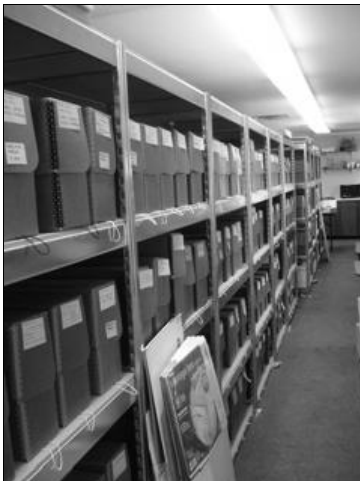
The weight of documents in these boxes are causing floor loading issues in Fuller Lodge. Photo by Christine Brown.
